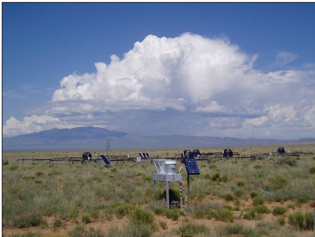
Figure 6 —Wet and dry deposition collector (foreground) and a long-term climate change experiment (background) in mixed species composition desert grassland in the Sevilleta National Wildlife Refuge. The climate change experiment is designed to determine the individual and interactive effects of increased winter precipitation, nighttime warming, and nitrogen deposition on this desert grassland ecosystem. Variables measured in each replicate (N = 5) are: air and soil temperature, soil moisture, plant available soil nitrogen, aboveground net primary production (ANPP), and plant species composition. In addition, a subset of the treatment also continuously measures soil respiration. See http://sev.lternet.edu/projects for more information on this and other climate change related research being conducted as part of the National Science Foundation-funded Sevilleta Long-Term Ecological Research Program. Photo credit: Sevilleta LTER Program.
